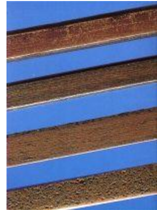
These photographs taken under a microscope show the differing wear characteristics to the overhead wire from using carbon, copper, sintered metal and aluminium as a collector material.
